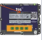
If the Sentry 600 gateway display shows the last report was within 10 minutes (screen shows Last: 10 min or less) and the display shows a connection with good signal strength (signal bars) it can be mounted at this location.
